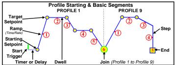
following a Start Trigger, profiles can start immediately, or if enabled after a dela or at a specified day & time (Recorder only).
