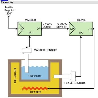
In this example the controlling actuator is a heater, indirectly heating the product via an oil jacket. The maximum input to the slave represents 300°C, thus restricting the jacket temperature. At start-up the master compares the product temperature (ambient) to its setpoint (250°C) and gives 100%. This sets the maximum slave setpoint (300°C), which is compared to the oil temperature (ambient) and the slave requests maximum heater output.
