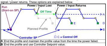
Continue profile from the point it had reached when the power failed On Recorder versions, option E will always be used if the power / signal is lost for less than the Profile Recovery Time. If the power / signal is lost for more than this time the defined Profile Recovery Method is used.
