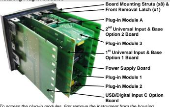
To access the plug-in modules, first remove the instrument from the housing. Pull front out to engage Front Latch. This prevents removal without a tool.
