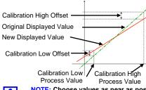
This example shows the effect of adding a positive Low Offset and a negative High Offset. E.a. if the process displays +0.0 at the low end, an offset of +0.5 would change the value to +0.5 A high end value of 100 with a 1.7 offset would read 98.3. There is a linear relationship between the two calibration points
