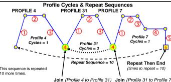
A profile can be made to run itself 1 to 9999 times or continuously using the Profile cycles setting. A profile ending with Repeat Then End will run the entire sequence of profiles again 1 to 9999 times or continuously.
